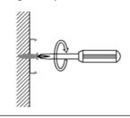
5. Mounting the fixture with clips
