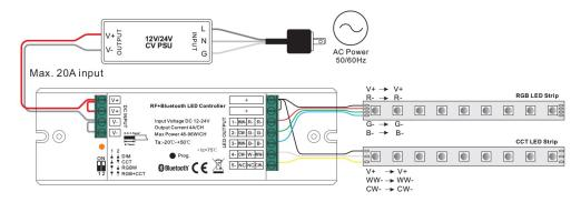
Note: please make sure the dial switches are at position for RGB+CCT mode as shown in above diagram.
