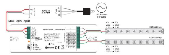
Note: please make sure the dial switches are at position for CCT mode as shown in above diagram.
