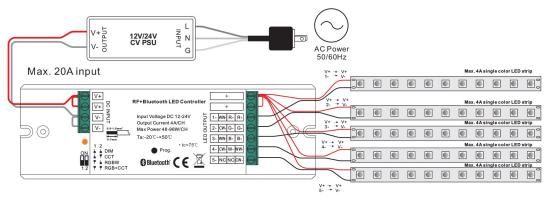
Note: please make sure the dial switches are at position for DIM mode as shown in above diagram.
